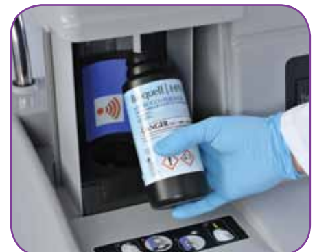
Image 3. Safe and secure bottle loading mechanism
